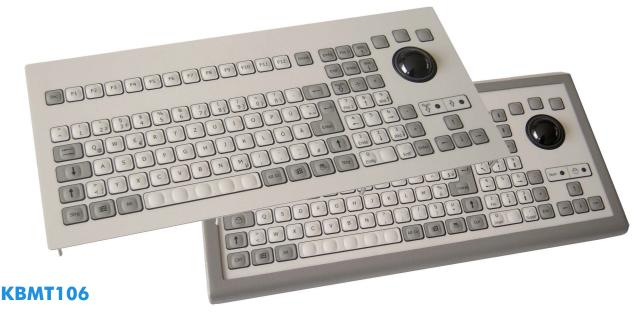
The unit features a full MF (multi-functional) keyboard with separate numeric-, cursor- and control keypads. The robust industrial grade trackball has a ball diameter of 38 mm and allows highest precision in cursor control. The keyboard part is sealed to IP65, the self-adjusting PTFE seal of the trackball enables an IP65 static (ball in rest) protection grade. Colour scheme and legend styling fit with the most recent industrial computer equipment.
