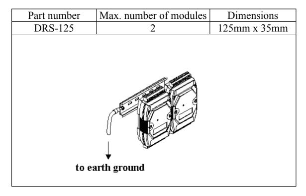
**Note**: It is recommended that a 16 - 14 AWG wire is used to connect the DIN rail to the earth ground.
