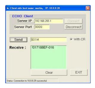
This TCP application uses the DCON Protocol to communicate with Ethernet port 9999 of the I-7188EF-016 Ethernet I/O controller.
