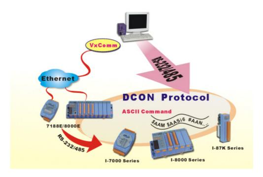
The DCON protocol is a request/reply communication protocol for the I-7000/8000/87K series I/O modules and I-7188EF-016, and uses a simple ASCII format such as \$AAN, \$AASi6, #AAN, #AASiCj, etc. The protocol format is defined as follows:
