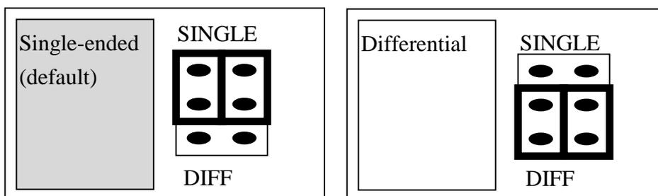
The A-821PGL/PGH offer 16 single-ended or 8 differential analog input signals. The JP3 select single-ended/differential. The user can not select single-ended and differential simultaneously.
