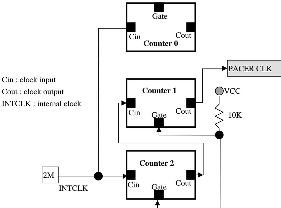
The counter1 and counter2 are all 16 bits counter. The counter 1 and counter 2 cascade as a 32 bits timer. This 32 bits timer is used as pacер timer. The software driver, `A-822_Delay()`,
