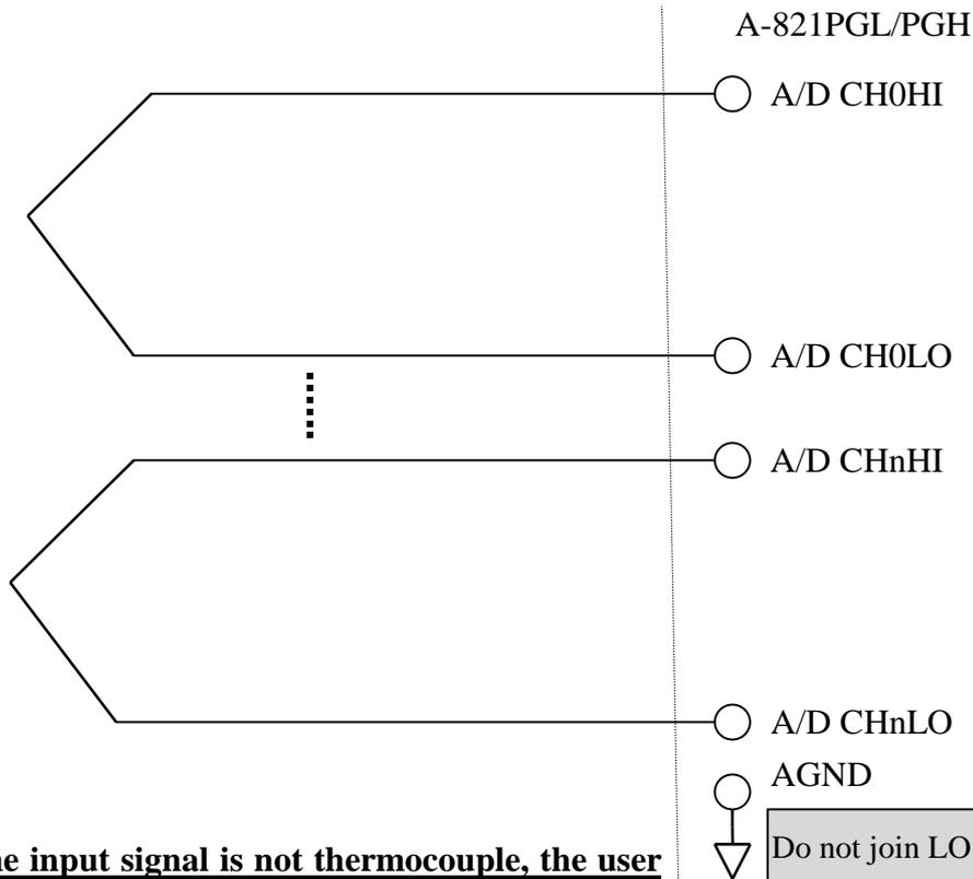
**Note : If the input signal is not thermocouple, the user should use oscilloscope to measure common mode voltage of  $V_{in}$  before connecting to A-821PGL/PGH.**
