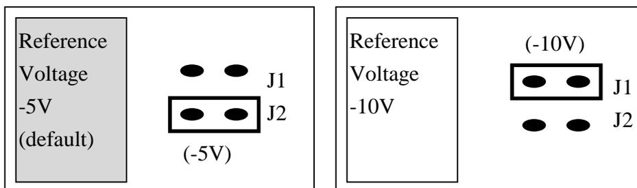
Select (-5V) : D/A voltage output = 0 to 5V (both channel)
