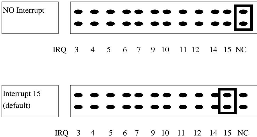
The interrupt channel **can not be shared**. The A826 software driver can support 8 different boards in one system but only **2 of these cards** can use interrupt transfer function.
