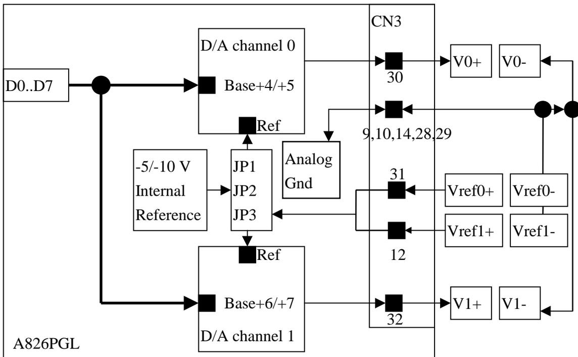
NOTE : The DA output latch registers are designed as “double buffer” structure. **The user must send the low byte data first, then send the high byte data to store the DA 12 bits digital data.** If the user only send the high byte data , then the low byte data will be still the previous value. Also if the user send high byte first then send low byte, the low byte data of DA is still hold in the previous one.
