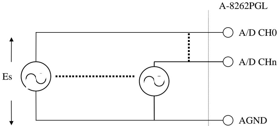
**FG3 : connecting to thermocouple input**
