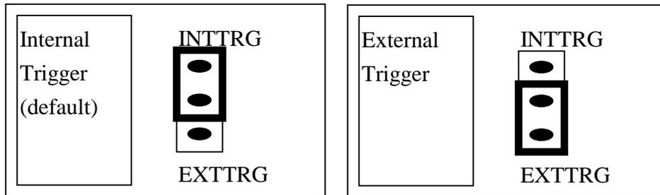
The A-826PG supports two trigger type, **internal trigger** and **external trigger**. The external trigger signal comes from **ExtTrg, CN3 pin 17**. There are two types of internal trigger, **software trigger** and **pacer trigger**.
