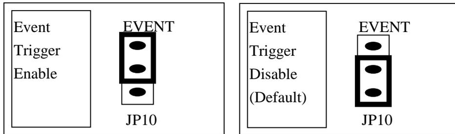
Both of the machine independent timer and the event trigger controller use timer/counter 0. Only one of these two function can be implemented. **So the user can not use both function at the same time.**
