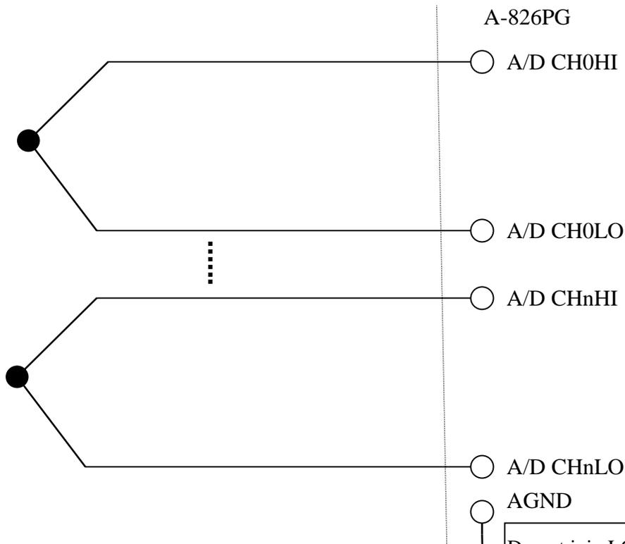
**Note : If the input signal is not thermocouple, the user should use oscilloscope to measure common mode voltage of Vin before connecting to A-826PG. Don't use voltage meter or multimeter.**
