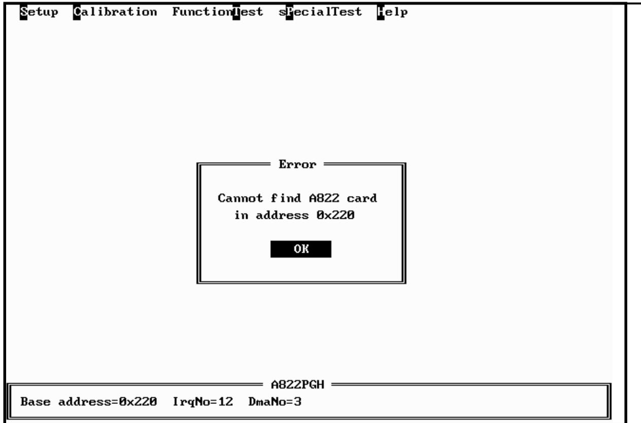
Although you can continue the A82XDIAG by press any key, it is recommended to correct this situation by setting the proper jumper setting. Because many operation in the A82XDIAG, the I/O base address is check firstly. And it don't work if the error occurs
