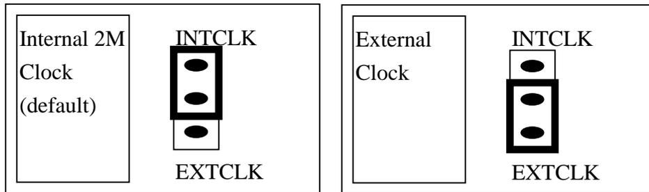
The A-826PG has 3 independent 16 bits timer/counter. The cascaded counter1 and counter2 are used as **pacemaker timer**. The counter0 can be used as a user programmable timer/counter. The user programmable timer/counter can select **2M internal clock** or **external clock ExtCLK, CN3 pin 37**. The block diagram is given in section 2.6. The clock source must be very **stable**. It is recommended to use internal 2M clock.
