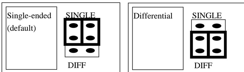
The A-826PG offer 16 single-ended or 8 differential analog input signals. The JP4 select single-ended/differential. The user can not select single-ended and differential simultaneously.
