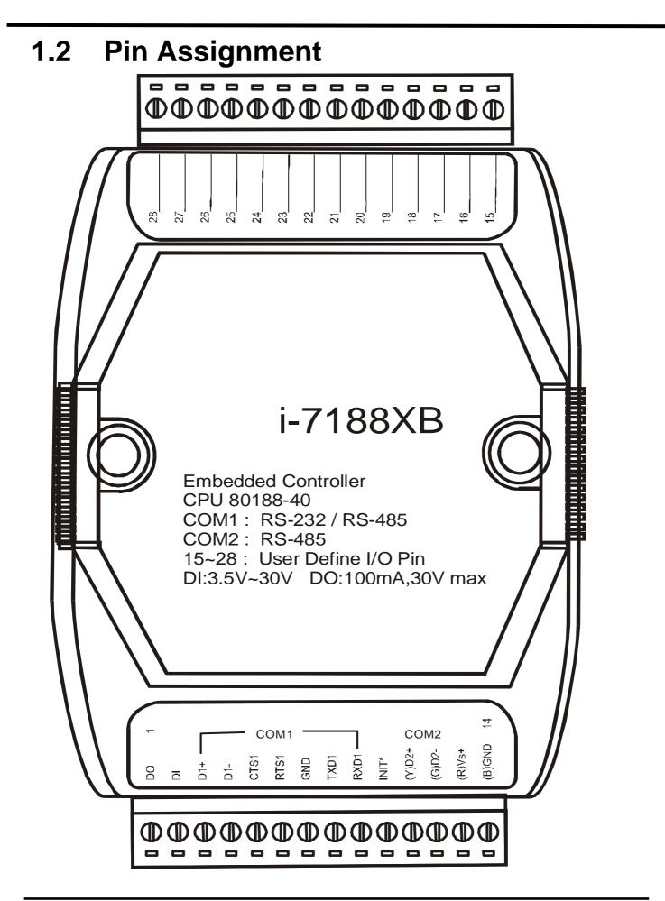
Pin assignment of bottom 14-pin screw terminal block(7188XB/7188XBD):
