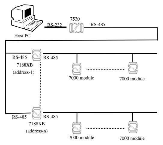
The 7000 series modules are slave devices; the control programs are implemented in host PC. The working steps are given as follows:
