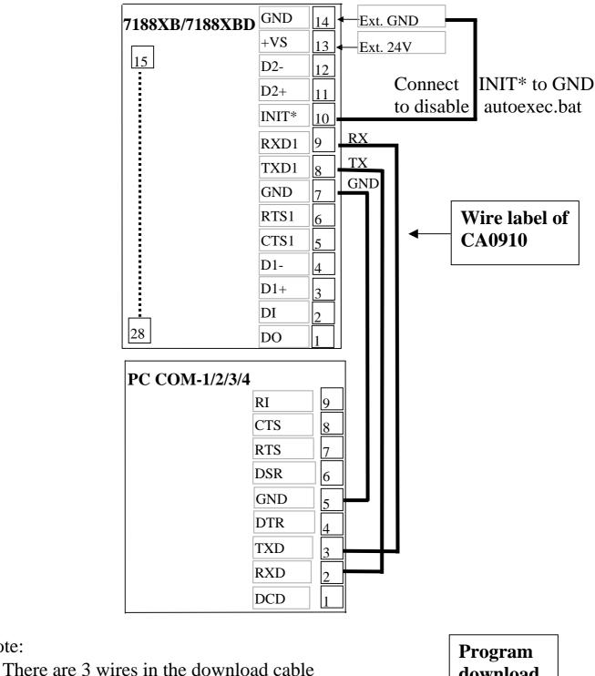
Connect the wire-1, label RX, to pin-8 of 7188XB •
