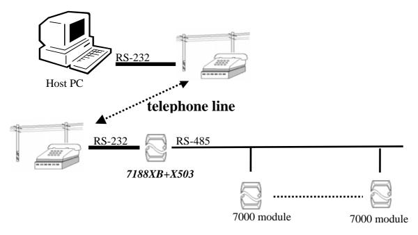
The control program is implemented in a local 7188XB. The 7188XB will directly control the 7000 modules based on these control arguments.
