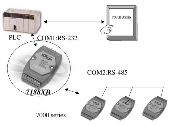
There is a Man Machine Interface in most PLCs. This interface is originally designed for MMI applications. The 7188XB can use this interface to build a bridge between PLC & 7000 modules.
