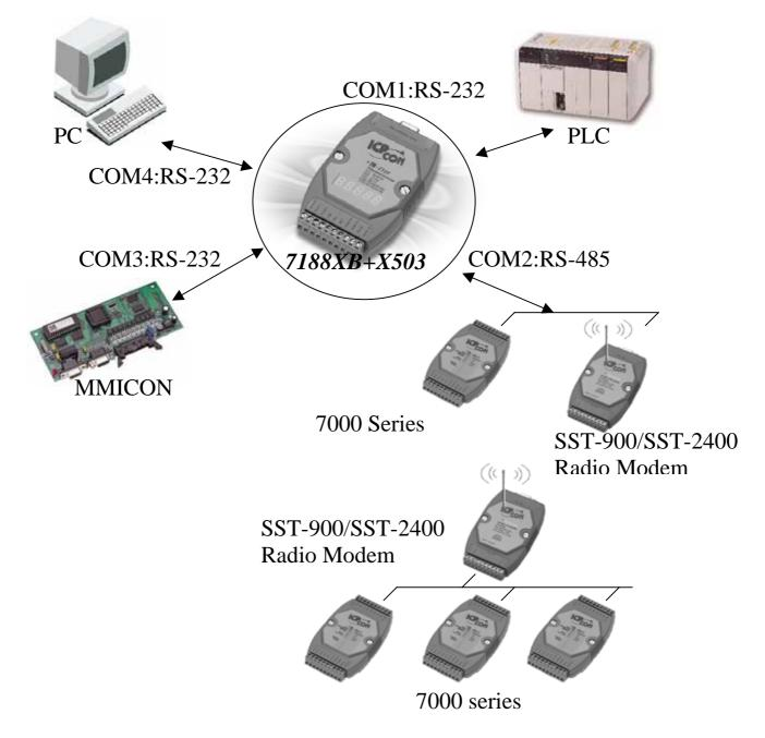
COM1: PLC can access the I/O states of 7000 modules COM2: Directly controls the 7000 input/output modules COM3: MMICON is used as the local MMI COM4: PC is used to monitor & record the system data.
