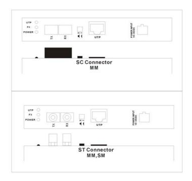
The Wavelength used is 850nm. The series also support MM(multimode)
