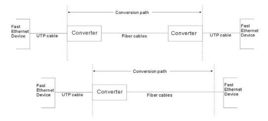
**Important rule :** When a connection is established, make sure the devices located at both ends of the path are configured and operated using the same duplex mode and the maximum distance must comply with IEEE 802.3u specifications.
