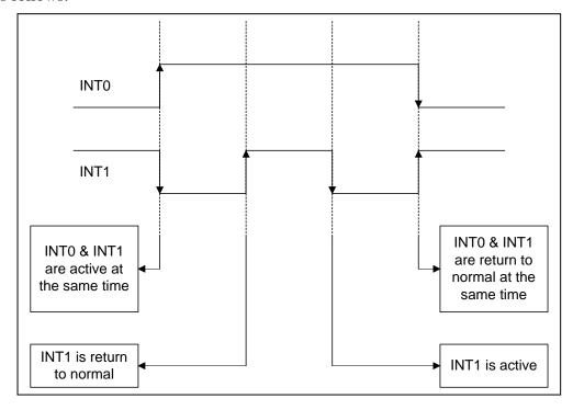
Refer to DEMO5.C for source program. **All of these falling-edge & rising-edge can be detected by DEMO5.C.**
