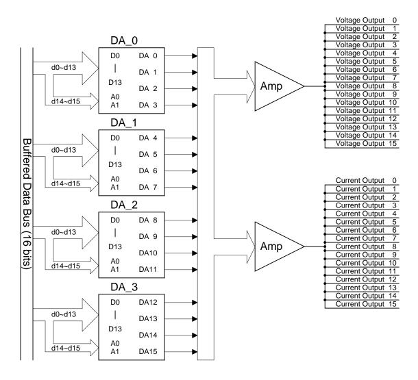
The PIO-DA16/8/4 offers 16/8/4 channels double-buffered digital to analog output and provide voltage output & current output simultaneous.
