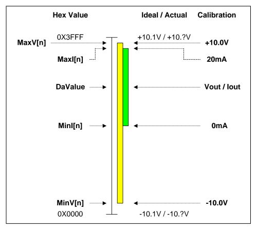
Therefore the software can calibrate the analog output without any hardware Trim-
