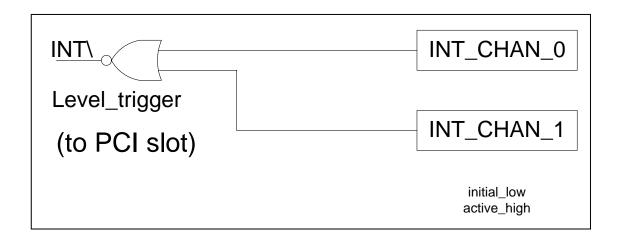
The interrupt output signal of PIO-DA16/8/4, INT\, is Level-Trigger & Active\_Low. If the INT\ generate a low\_pulse, the PIO-DA16/8/4 will interrupt the PC once a time. If INT\ is fixed in low\_level, the PIO-DA16/8/4 will interrupt the PC continuously. So the INT\_CHAN\_0/1 must be controlled in a pules\_type signals. They must be fixed in low\_level statue normally and generated a high\_pulse to interrupt the PC.
