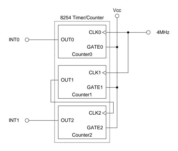
It provides two interrupt source, one is 16 bits timer output (INT0) and the other one is 32 bits timer output (INT1).
