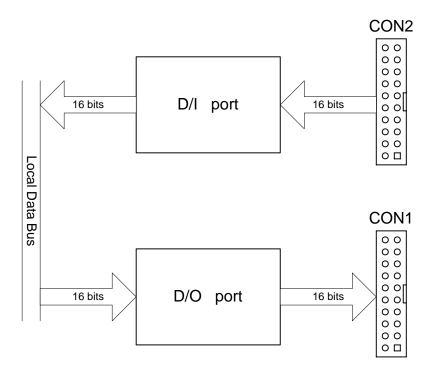
The D/I port can be connected to the DB-16P. The DB-16P is a 16 channels isolated digital input daughter board. The D/O port can be connected to the DB-16R or DB-24PR. The DB-16R is a 16 channels relay output board. The DB-24PR is a 24 channels power relay output board.
