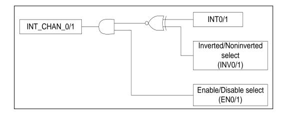
The architecture of INT\_CHAN\_0 and INT\_CHAN\_1 is the same as above figure. The only difference between INT0 and INT1 is that INT\_CHAN\_0 signal source from 8254 counter0 output and INT\_CHAN\_1 signal source from 8254 counter2 output.
