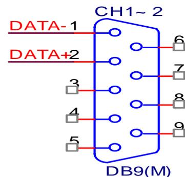
**Warning:** The RS-485 bus is a differential (balanced) signal, thus **you cannot wire the Data+ with Data- directly for a single port loop-back test.** It will not work at all!
