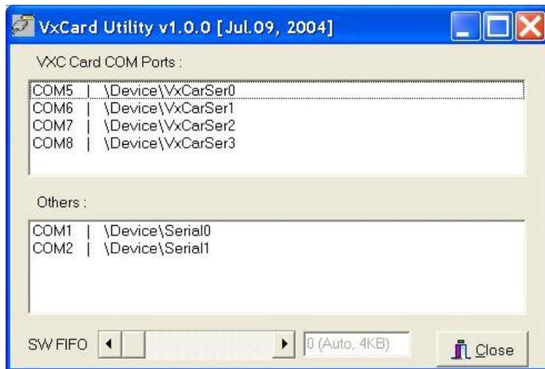
To change the COM port mappings, users should restart the driver by rebooting the computer, or re-install the “**VXC Card**” hardware in the “**Device Manager**” by un-install card and then scan new hardware.
