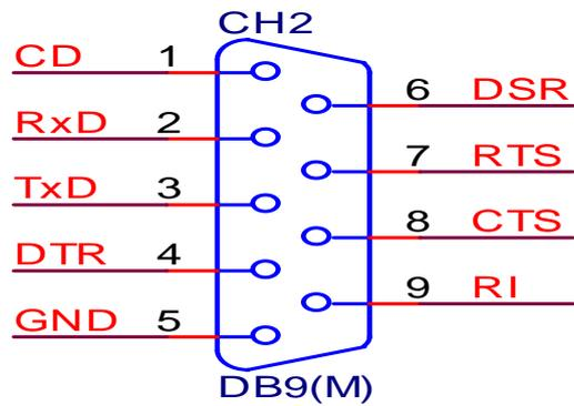
VXC-112A, VXC-182i (Male DB-9) Null Modem Cable Wiring
