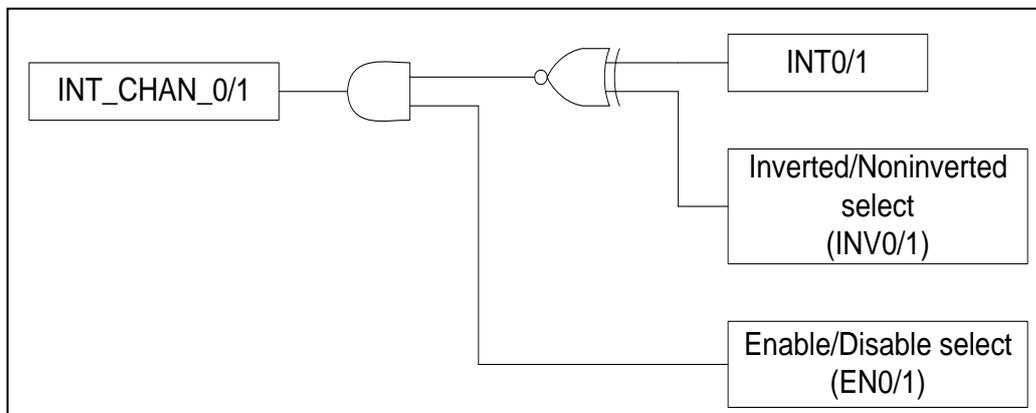
The INT\_CHAN\_0 and INT\_CHAN\_1 architecture is shown in the above figure. The only difference between INT0 and INT1 is that the INT\_CHAN\_0 signal source comes from the UART 0 interrupt output, and the INT\_CHAN\_1 signal source comes from the UART 1 interrupt output.
