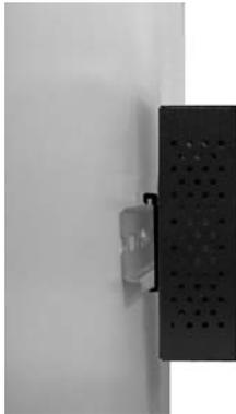
3. Check if the DIN-Rail is tightened on the track or not.
