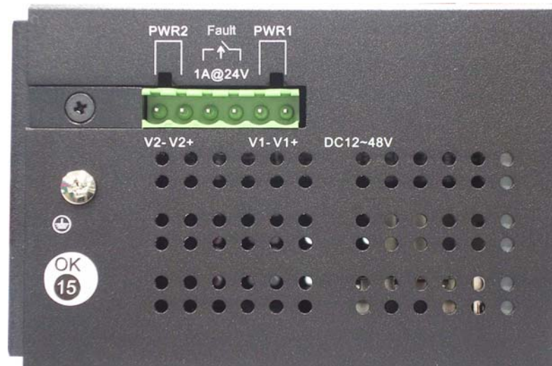
Top Panel of the industrial switch
