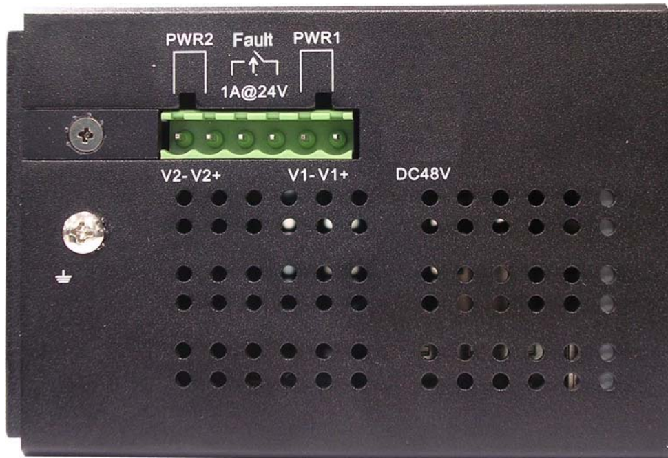
Top View of the PoE Injectors Industrial Switch
