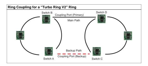
The "Coupling Port (Backup)" on Switch A is used for the backup path, and connects directly to an extra network port on Switch C. The "Coupling Port (Primary)" on Switch B monitors the status of the main path, and connects directly to an extra network port on Switch D. With ring coupling established, Switch A can activate the backup path as soon as it detects a problem with the main path.
