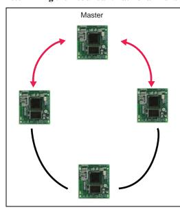
For a "Turbo Ring V2" ring, the backup segment is the segment connected to the 2nd redundant port on the master.
