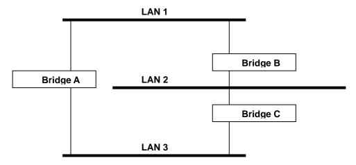
If STP is enabled, it will detect duplicate paths and prevent, or *block*, one of them from forwarding traffic. In the following example, STP determines that traffic from LAN segment 2 to LAN segment 1 should flow through Bridges C and A as this path has a greater bandwidth and is therefore more efficient.
