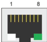
The LED indicator in the lower right corner glows a solid green color when the cable is properly connected to a 100 Mbps Ethernet network. The LED will flash on and off when Ethernet packets are being transmitted or received.
