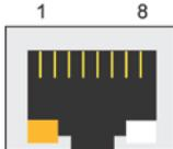
The LED indicator in the lower left corner glows a solid orange color when the cable is properly connected to a 10 Mbps Ethernet network. The LED will flash on and off when Ethernet packets are being transmitted or received.
