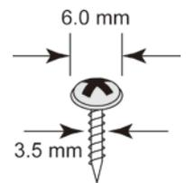
**NOTE** Before tightening the screws into the wall, make sure the screw head and shank size are suitable by inserting the screw into one of the keyhole-shaped apertures of the Wall Mounting Plates.
