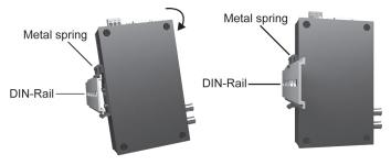
To remove the ICF-1170I series from the DIN-Rail, simply reverse Steps 1 and 2 above.
