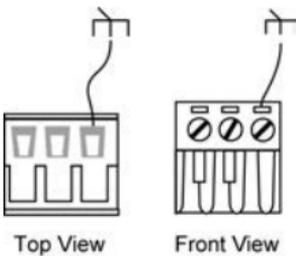
Grounding and wire routing help limit the effects of noise due to electromagnetic interference (EMI). Run the right most contact of the 3-contact terminal block to the grounding surface prior to connecting devices.
