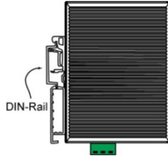
To remove the INJ-24 from the DIN-Rail, insert a flat-blade screw driver horizontally into the DIN-Rail kit under the INJ-24, and then pull it upwards and release INJ-24 towards you away from the DIN-Rail.
