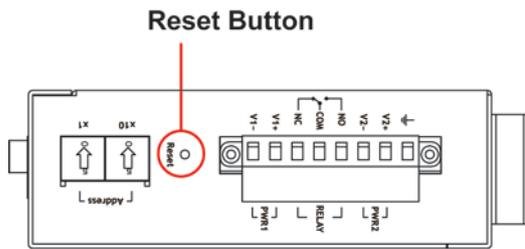
To reset the MGate to the factory default settings, hold down the reset button for about 5 seconds. The MGate will restart and be reset to factory default settings.
