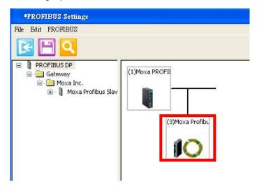
To remove the device from the PROFIBUS network in the right top panel, users can click the device and press the delete key.
