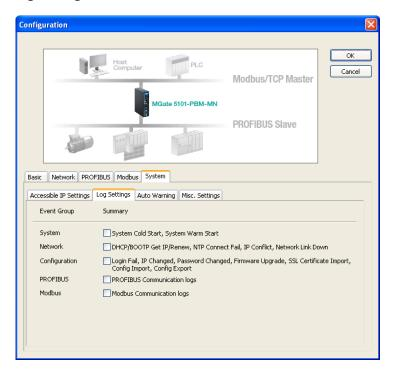
This setting will enable the MGate firmware to record the important event for future verification. The record information can only be displayed in web console. Please refer to chapter 5.
