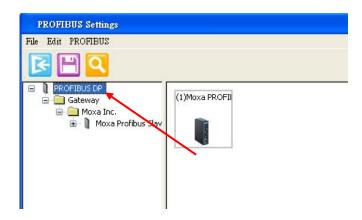
To add the device into the PROFIBUS network in the right top panel, users can use mouse the drag the device into the right panel. And user will also see the device lists in the right bottom panel.
