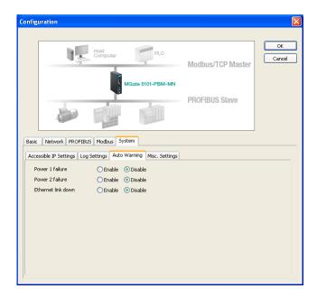
Auto Warning will be triggered in the event of a power failure or when Ethernet links are disconnected. When a checked trigger condition occurs, the MGate will open the circuit of the relay output and trigger the Fault LED to start blinking. Otherwise, the MGate will short circuit the relay output.
