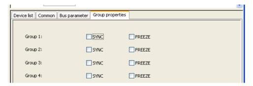
SYNC: In data\_exchange the previous output value will be transferred. The following output data will be stored and not be transferred until next SYNC command or UNSYNC command.
