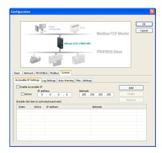
This settings is used this restrict access to the module by IP address. Only IP addresses on the list will be allowed access to the module. You may add a specific address or range of addresses by using a combination of IP address and netmask, as follows:
