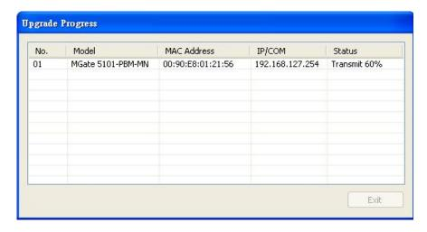
Once the firmware has been successfully written onto the unit, click **Exit** to close the Upgrade Firmware window. MGate Manager will automatically execute a Broadcast Search for all MGate units on the LAN. Your MGate should reappear in the list of units.
