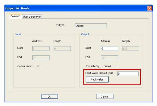
In some application, users want to define how to deal with the PROFIBUS output when Modbus TCP side doesn't work well. This is defined as the "Fault value". In MGate, it provides a setting for each PROFIBUS I/O module to handle such situation.
