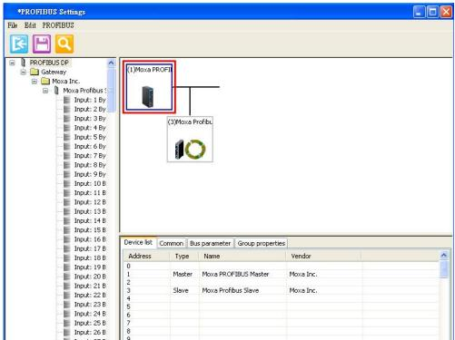
Step 5: Configure the I/O module for the target PROFIBUS slave device which users want to access.
