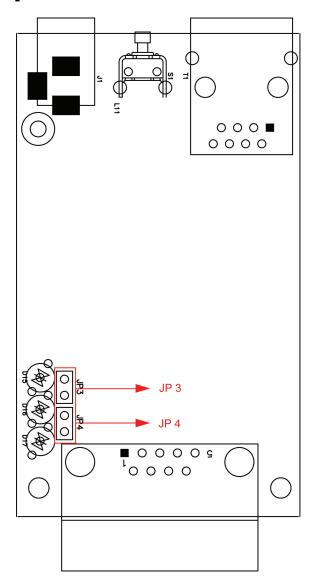
To set the pull high/low resistors to 150 K $\Omega$ , leave jumpers JP3 and JP4 open (not shorted). This is the default setting.
