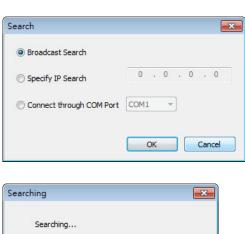
When the search is complete, every MGate MB3000 that is found on the LAN will appear in the window with MAC address and IP address. Simply select the one that you wish to configure.
