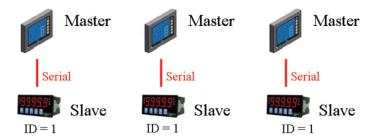
The MGate MB3000 can connect to each serial slave so Ethernet SCADA masters will be able to control them. However, since slave IDs cannot be repeated in a system, we will need to change the IDs of some of the slaves in order to integrate them into a single network, as follows:
