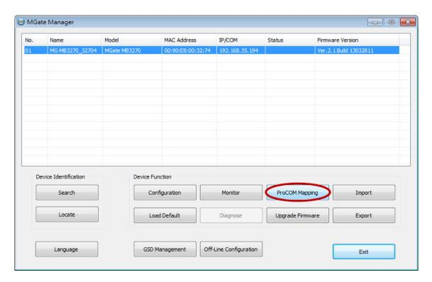
On the ProCOM mapping dialog box, you can map up to four ProCOM functions for each Modbus gateway to your PC's COM ports. The driver will generate virtaul COM ports on your PC to connect to the selected MGate MB3000s over the network.
