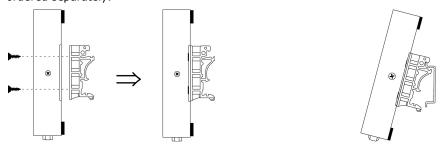
**Mounting on the wall:** You will first need to attach the mounting plates to the unit. Place four screws in the wall and slide the unit onto the screws as shown.
