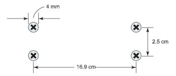
The head of each screw should be 6 mm or less in diameter, and the shaft should be 3 mm or less in diameter. Make sure to leave about 5 mm of space between the head and the wall.
