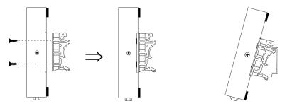
**Mounting on the wall:** Place two screws in the wall and slide the unit onto the screws as shown. The head of each screw 6.5 mm or less in diameter, and the shaft should be 3 mm or less in diameter. Make sure to leave about 2 mm of space between the head and the wall.
