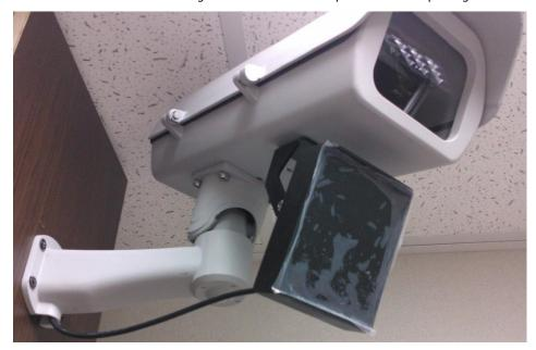
**NOTE** Be sure to install the VP-IR2 onto the VP-CI701 housing and VP-CI800 bracket before you install it on the wall.
