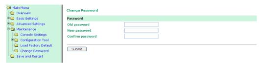
Enter the old password and new passwords and click on Submit. To remove password protection, leave the new password blank and just enter the old password.
