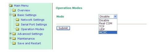
After **MCSC mode** is selected, you will see 2 channels that are ready to configured. Under the MCSC structure, each channel works independently so you need to configure each channel separately according to your application. Click **Modify** to configure the Channel 1.
