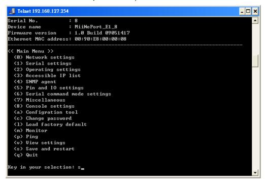
9. Press **Y** and then **Enter** to save the new IP address and restart the module.
