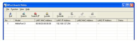
4. To modify the configuration of the highlighted MiiNePort E1, click the **Console** icon to open the web console. This will take you to the web console, where you can make configuration changes. Refer to **Chapter 7:** Web Console Configuration for information on how to use the web console.
