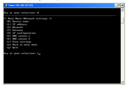
5. Use the Backspace key to erase the current IP address. Type in the new IP address and then press **Enter**.
