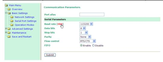
MiiNePort E1 supports the **Any Baud Rate (non-standard baud rate)** feature. If your baud rate is not listed, select **Other** from the drop-down list and type the baud rate in the input box. MiiNePort E1 will use the closest baud rate we can support.
