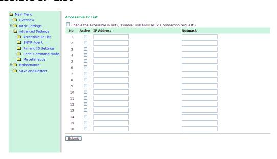
· To allow access to a specific IP address
