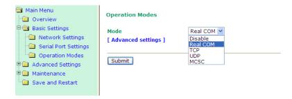
Before reading this section, refer to **Chapter 3: Choosing the Proper Operation Mode** to select the operation mode that best fits your device application.
