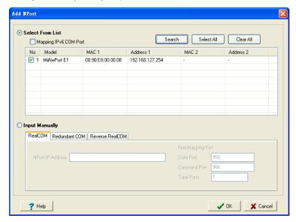
4. Alternatively, you can select Input Manually and then manually enter the MiiNePort E1 module's IP Address, 1st Data Port, 1st Command Port, and Total Ports to which COM ports will be mapped. Click OK to proceed to the next step. Note that the Add NPort page supports FQDN (Fully Qualified Domain Name), in which case the IP address will be filled in automatically.
