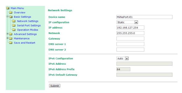
You must assign a valid IP address to the module before it will work in your network environment. Your network system administrator should provide you with an IP address and related settings for your network. The IP address must be unique within the network; otherwise the module will not have a valid connection to the network. First time users can refer to **Chapter 5: Initial IP Address Configuration** for more information.
