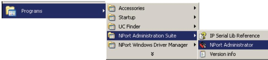
2. Unlock the NPort 5000AI-M12 you wish to configure if it is password protected. Right click a specific NPort 5000AI-M12 and select the **Upgrade Firmware** function to start upgrading the firmware.
