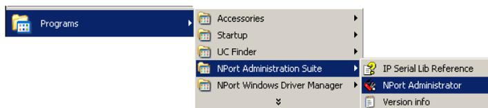
2. Unlock the NPort 5000AI-M12 you wish to configure if it is password protected. Right click the NPort 5000AI-M12 and select Configure to start the configuration.
