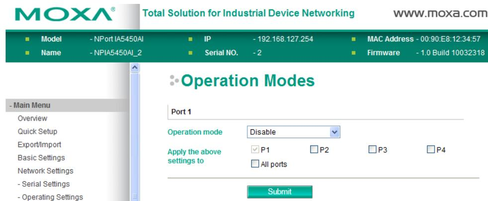
When Operation mode is set to Disabled, that particular port will be disabled. Check the “Apply the above settings to all serial ports” to apply this setting to the other port.
