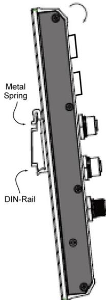
**STEP 3:** Swing the device server down fully onto the DIN-Rail until both clamps completely latch.
