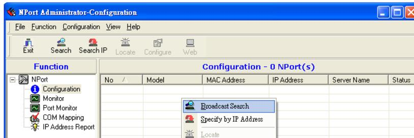
2. The **Broadcast Search** window will open and display the Model, IP Address, MAC Address, and Progress of the search for that particular device.
