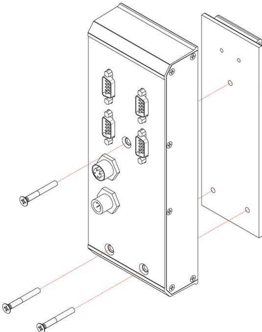
**STEP 2:** Position the NPort 5000AI-M12 on the DIN-Rail, tilting to hook clamps over the top edge of the rail.
