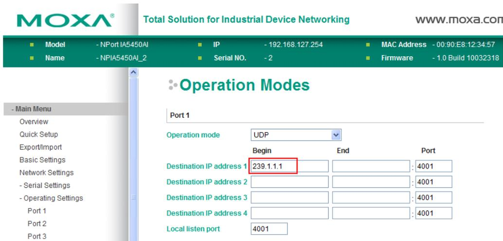
To add a network host to the multicast group, input the host’s IP address (e.g., 239.1.1.1) in one of the **Destination IP address** input boxes, as illustrated above. The NPort will automatically add this host to the multicast group, and the host will start receiving all packets sent by the NPort to this group.
