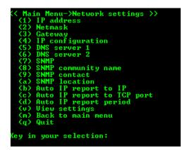
6. Use the Backspace key to erase the current IP address, type in the new IP address, and then press Enter.
