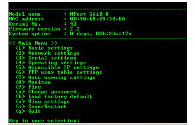
10. Type y or Y and then press Enter to save the new IP address and restart NPort.
