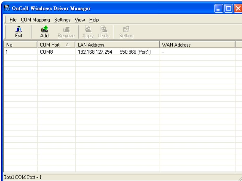
For Reverse Real COM mode, you can select **Input Manually** and then manually enter the LAN MAC address for OnCell G3111/G3151/G3211/G3251. Click **OK** to proceed to the next step.
