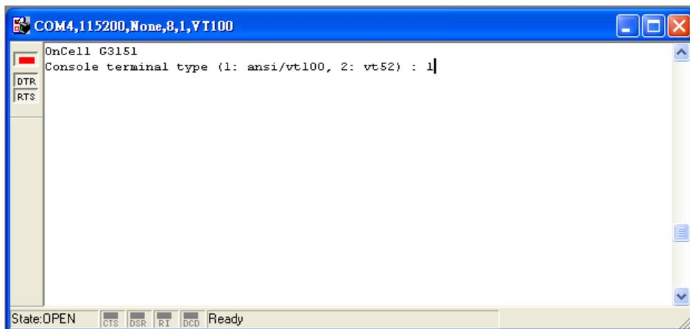
8. The main menu should appear. Once you are in the console, you may configure the IP address through the **Network** menu item, just as with the Telnet console. Please refer to steps 4 to 11 in the **Telnet Console** section to complete the initial IP configuration.
