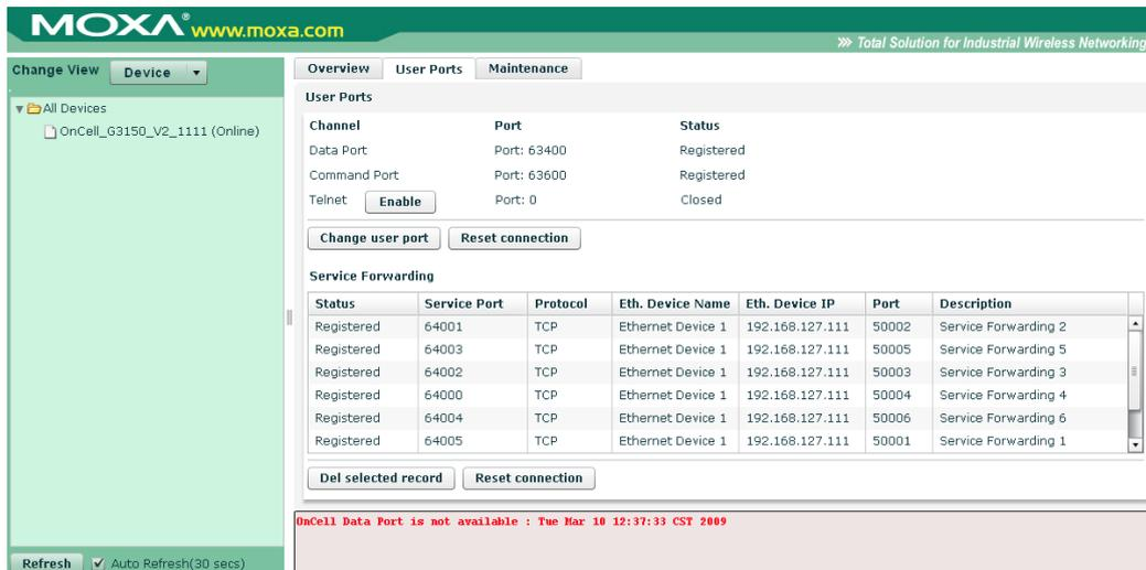
**Note:** If the data or command port is occupied, an error message will appear at the bottom of the window.
