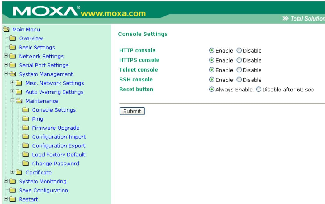
On this screen, access to different OnCell G3111/G3151/G3211/G3251 configuration console options (HTTP, HTTPS, Telnet, SSH) can be enabled or disabled. Please refer to Change Password later in this chapter for more information on passwords. Finally, you may also enable or disable the reset button.
