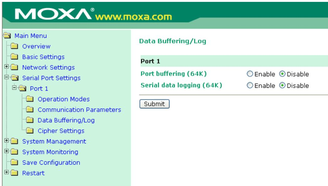
The OnCell G3111/G3151/G3211/G3251 supports port buffering to prevent the loss of serial data when the Cellular or Ethernet connection is down. Port buffering can be used in Real COM, Secure Real COM, Reverse Real COM, Secure Reverse Real COM, RFC2217, TCP Server, Secure TCP Server, TCP Client, Secure TCP Client, and SMS Tunnel modes. For other modes, the port buffering settings will have no effect.
