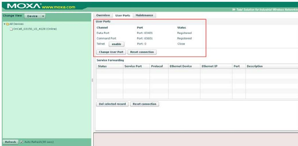
**Telnet Enable:** If you click on the enable icon, this mean the telnet is enable for host to connect to OnCell device.
