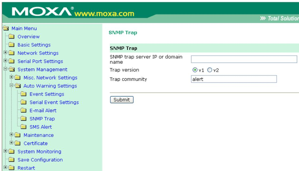
**SNMP trap server IP:** Use this field to indicate the IP address to use for receiving SNMP traps.
