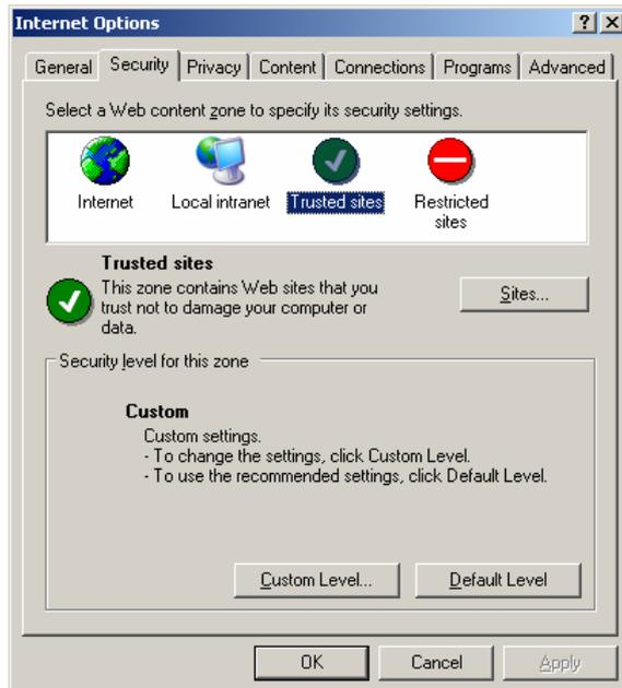
2. In either case, the window below should appear, showing the list of sites that you have configured Internet Explorer to trust. Add the IP address of your OnCell G3111/G3151/G3211/G3251 here (the factory default IP address is 192.168.127.254).
