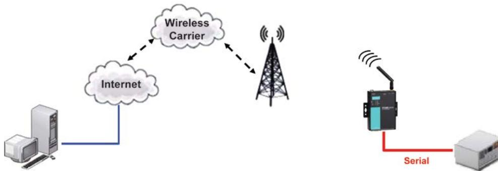
The OnCell G3111/G3151/G3211/G3251 cellular IP gateway enables traditional serial (RS-232/422/485) devices for transmitting data over the cellular network. The IP gateway is a tiny computer equipped with a CPU and TCP/IP protocols that can bi-directionally translate data between the serial and IP formats. With the OnCell G3111/G3151/G3211/G3251, your computer will be able to access, manage, and configure remote facilities and equipment over the cellular network from anywhere in the world.
