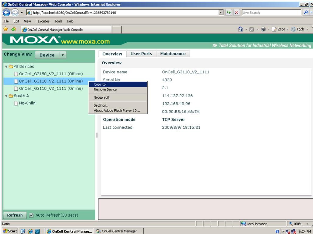
**Remove Device.** To maintain the list, you can remove all offline devices. To activate this function, **click the right mouse button and select Remove Device.**
