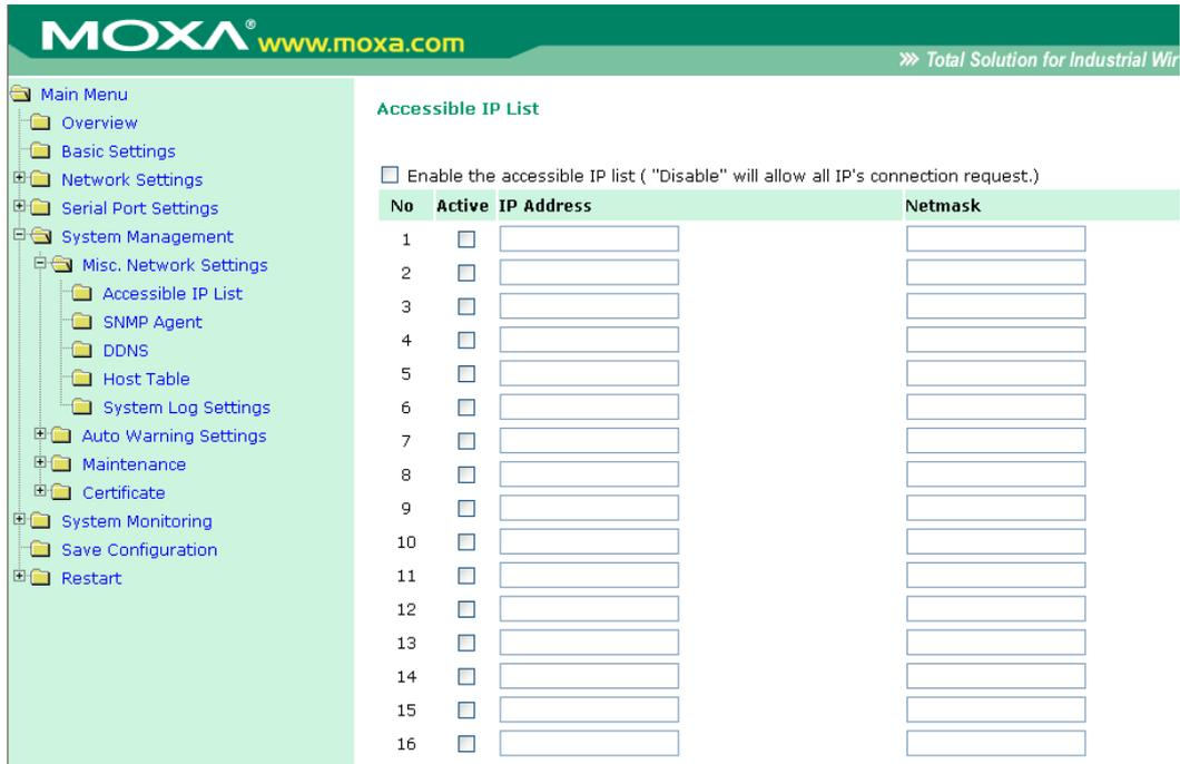
The OnCell G3111/G3151/G3211/G3251 uses an IP address-based filtering method to control access to its serial ports.
