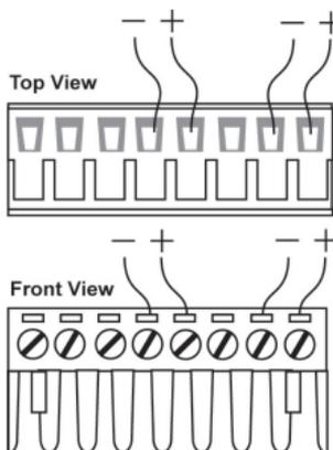
**STEP 1:** Insert the negative/positive DC wires into the V-/V+ terminals.
