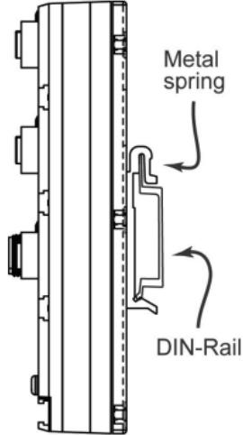
To remove the switch from the DIN-Rail, simply reverse Steps 2 and 3 above.
