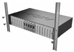
7. Install two (2) screws through the bracket at each side into the mounting rail, using the clip nuts to secure, if necessary.
