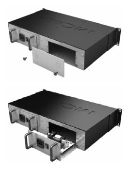
3. Where there is no plate on the chassis, slide the power supply module slowly and follow the installation guide in the chassis. Push the power supply module into the chassis till the end and ensure that the power supply module is firmly connected to the chassis.
