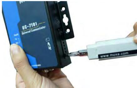
**Step 2:** After removing the cover, insert the SD memory card into the slot.
