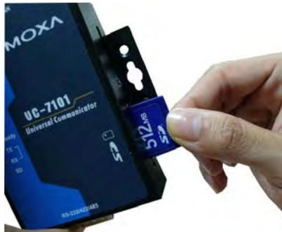
**NOTE:** To remove the SD card from the slot, press the SD card in slightly forward with your finger, and then remove your finger to cause the card to spring out partially. You may now grasp the top of the card with two fingers and pull it out.
