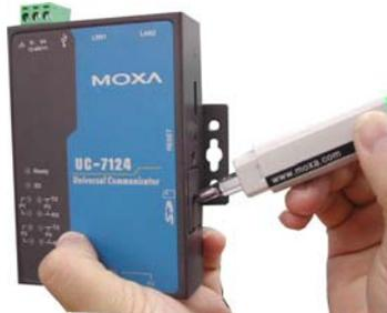
**Step 2:** After removing the cover, insert the SD memory card into the slot.
