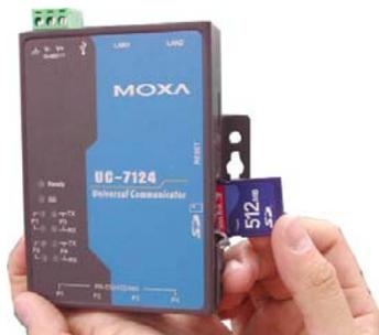
**NOTE:** To remove the SD card from the slot, press the SD card in slightly with your finger, and then remove your finger to cause the card to spring out partially. You may now grasp the top of the card with two fingers and pull it out.
