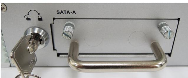
3. Pull out the faceplate by unscrewing the thumbscrews in the upper corners, and then remove the plate. Fasten the storage drive to the faceplate flange as shown below, using the two flathead screws that were shipped with your V2616A.
