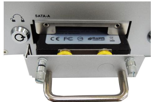
5. When finished, turn the key clockwise to activate the lock and tighten the thumbscrews. Use the same method to install a hard disk in second storage tray.
