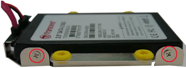
4. Install the storage kit into the V2616A computer. Fasten four screws on the kit, and connect the cable the power onto the V2616A's main board.
