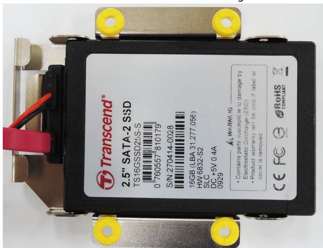
3. Fasten the two screws on each side of the hard disk (total of four).
