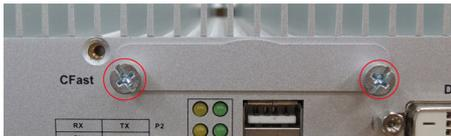
3. Insert the CFast card into the socket. Make sure you insert it in the correct direction. When finished, fasten the socket cover with screws.
