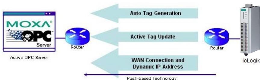
The "push" technology also includes the update for the tags. When the I/O status changes, the ioLogik will send updates to the Active OPC Server. Compared to polling the status (the so-called pull-based method), this feature efficiently reduces network bandwidth usage and speeds up response time with event-driven, push-based status updates. At the same time, the heartbeat function monitors the system's basic signs of life.
