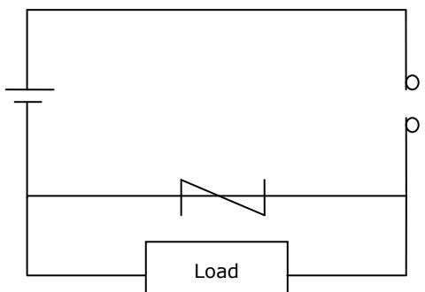
**NOTE** A "load" in a circuit schematic is a component or portion of the circuit that consumes electric power. For the diagrams shown in this document, "load" refers to the devices or systems connected to the remote I/O unit.
