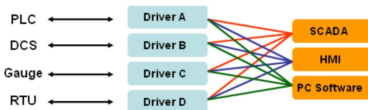
**OPC Client/Server creates a common interface to connect to different devices**
