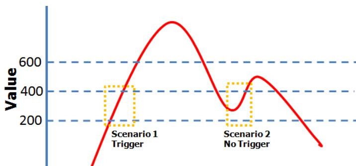
When Trigger = Smaller, Value = 400, and Hysteresis = 200, the SNMP trap will only be triggered if the RTD signal fluctuates from 600 to 400, as depicted in Scenario 1 below. However, if we change the settings to Value = 400 and Hysteresis = 400, the SNMP trap will only be triggered if the RTD signal fluctuates from 800 to 400.
