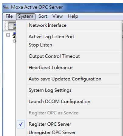
**Network Interface:** Select which network to use if the PC has multiple network adaptors installed.
