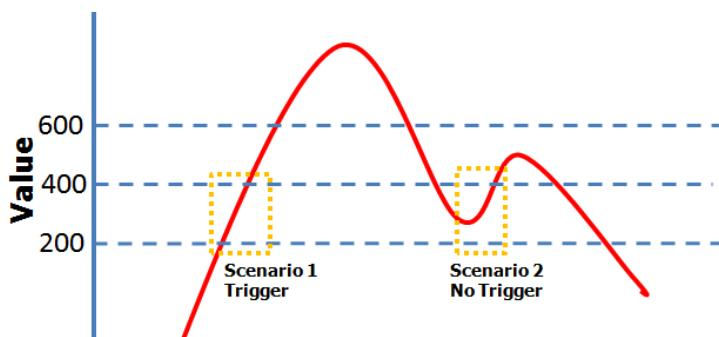
When Trigger = Smaller, Value = 400, and Hysteresis = 200, the SNMP trap will only be triggered if the TC signal fluctuates from 600 to 400, like in scenario 1. If we change to Value = 400 and Hysteresis = 400, the SNMP trap will only be triggered if the TC signal fluctuates from 800 to 400.
