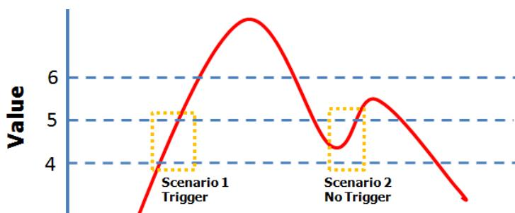
When Trigger = Smaller, Value = 5, and Hysteresis = 1, the SNMP trap will only be triggered if the analog signal fluctuates from 6 to 5, as depicted in Scenario 1 below. However, if we change the settings to Value = 5 and Hysteresis = 2, the SNMP trap will only be triggered if the analog signal fluctuates from 7 to 5.
