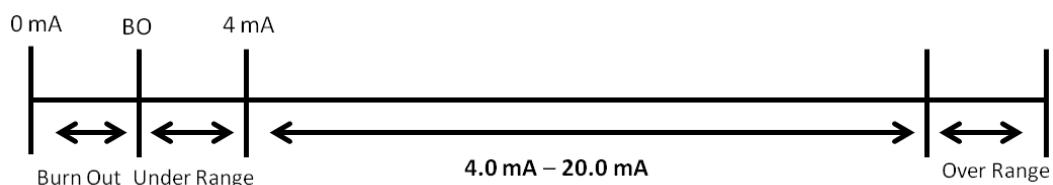
Users can define **Burn Out** (BO) values (default = 2 mA) for selected ranges. When input values are in the **Burn Out** range, raw data will register as 0000h to indicate that the analog input has burned out. The definition of raw data is as follows:
