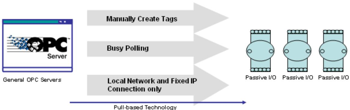
In addition, Moxa's ioLogik products now support OPC technology. An ioLogik can automatically generate tags without requesting any data or even a device's IP address. All the user needs to do is launch Active OPC Server, and the I/O channels selected by the user will be "pushed" from the ioLogik to Active OPC Server.
