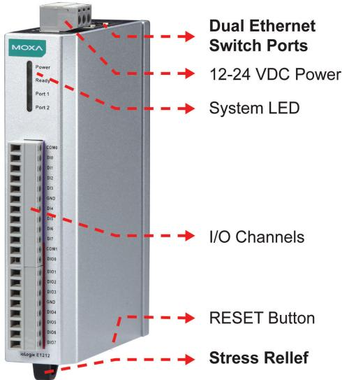
**NOTE** The RESET button restarts the server and resets all settings to factory defaults. Use a pointed object such as a straightened paper clip to hold down the RESET button for 5 seconds. The factory defaults will be loaded once the READY LED turns green again. You may then release the RESET button.
