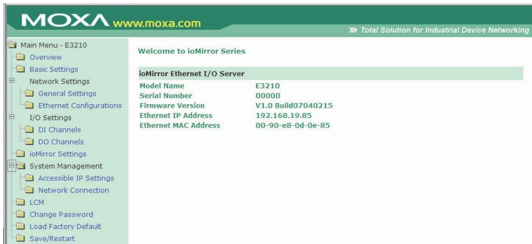
The main page of the web console displays detailed information about your ioMirror unit, including module name, serial number, firmware version, IP address, and MAC address.
