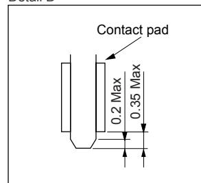
(All dimensions are in millimeters with  $\pm 0.15\text{mm}$  tolerance unless specified otherwise.)
