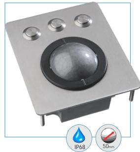
The TSX series are waterproof and vandalproof industrial trackball units and uses the latest generation of laser trackballs. These trackballs are highly suited for harsh industrial environments thanks to their robustness and ease of maintenance. They feature a removable top ring facilitating the cleaning of ball and ball compartment for use in even the most dusty environments. The concept itself of these laser trackballs make them waterproof as well.
