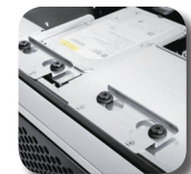
Anti-vibration drive cage design
