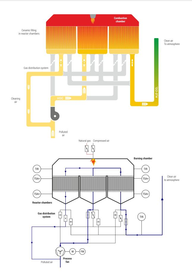
The purpose of the recuperative catalytic combustion is to purify gases (usually the polluted air mass) from volatile organic compounds (VOC).
