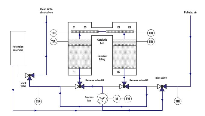
The purpose of the RTO is to purify the polluted air mass from volatile organic compounds (VOC) through direct combustion (oxidation).
