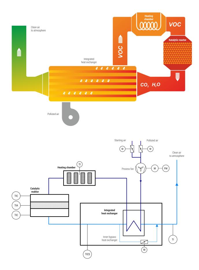
The purpose of the recuperative thermal oxidation is to purify gases (usually the polluted air mass) from volatile organic compounds (VOC) using direct combustion.
